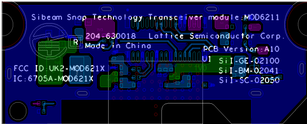
Figure 4.4. MOD6211 Transceiver Module Layout Floorplan
