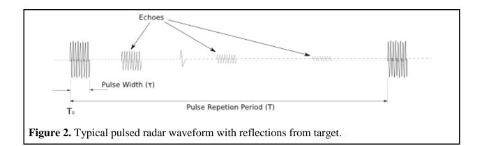
To calculate the wavelength ( $\lambda$ ), the speed of light (3 x 10^8 meters/second) will be denoted by "c" and the radar frequency "f" to gain the equation  $\lambda$  = c / f . By denoting "t" as the measured round trip propagation time, the radar range equation is r = (c \* t) / 2. The basic radar equation
